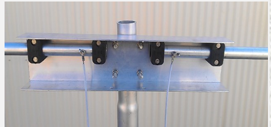
Leads showing the manner of attaching feed-wires on the 5mm studs with wing nuts.
